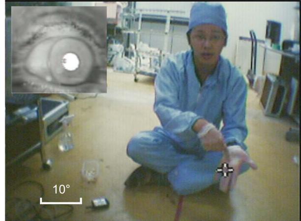
**Figure 1. Experimental apparatuses.** The eye tracker on Pan's head (A) and the eye (left top) and scene-camera image (B). Cross mark indicates point-of-regard (POR). Also, see Video S2. doi:10.1371/journal.pone.0059785.g001
